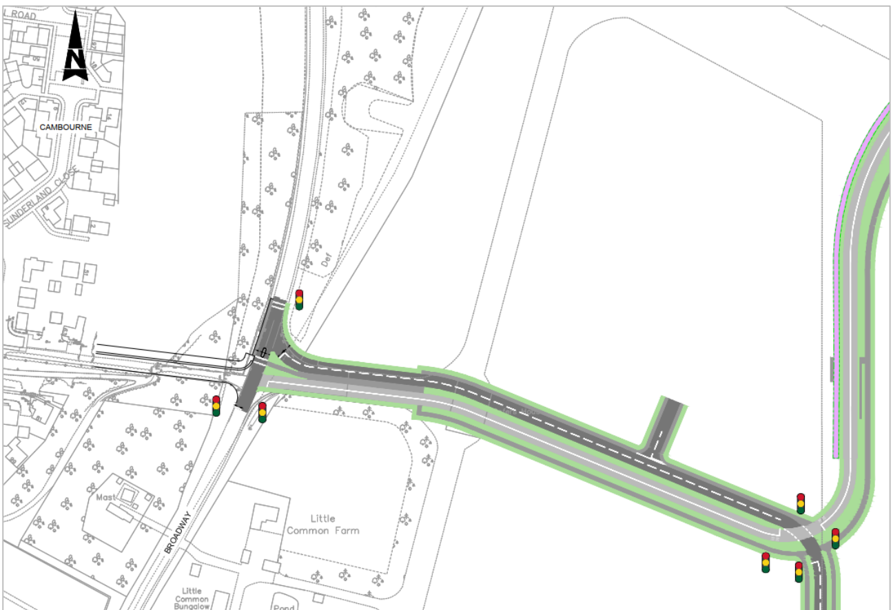
Figure 19: Technical drawing showing junction on Broadway with Bourn Airfield western access point (from OAR Part 3, page 70)
